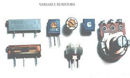
Figure 8. Some types of Variable resistances
